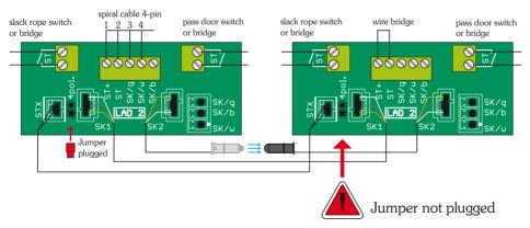
Note 1: When the jumper is used in the connection box, the slack rope switches/pass door switches are bridged in the main connection box.
