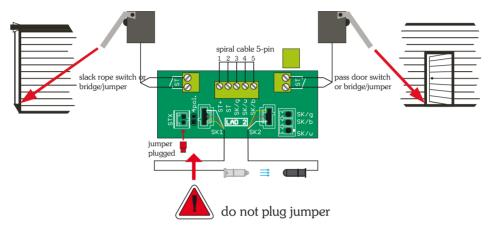
Note 2: If a jumper is used in connection with a 5-pin helix cable, the control is at risk of a short circuit. Use only with a 4-pin helix cable.
