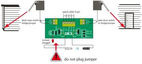
Note 2: If a jumper is used in connection with a 5-pin helix cable, the control is at risk of a short circuit. Use only with a 4-pin helix cable.
