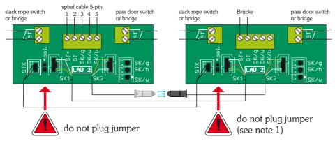
Note 2: If a jumper is used in connection with a 5-pin helix cable, the control is at risk of a short circuit. Use only with a 4-pin helix cable.
