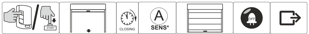
PUSH START DOOR CLOSING WAIT CLOSED DOOR DETECTED CLOSED DOOR LED OFF SAVE & QUIT
