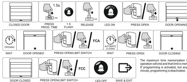
The maximum time memorization is 2 min. After which, the operation will end and that limit is memorized.
