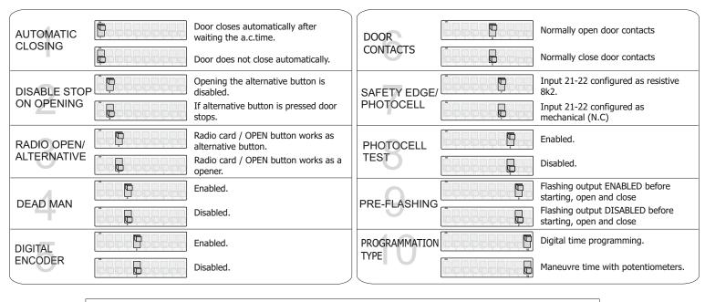
If OPTION 3 & 4 ON, control unit makes a normal opening and dead man on closing If OPTION 3 ON & OPTION 4 OFF, control unit makes dead man on opening and closing
